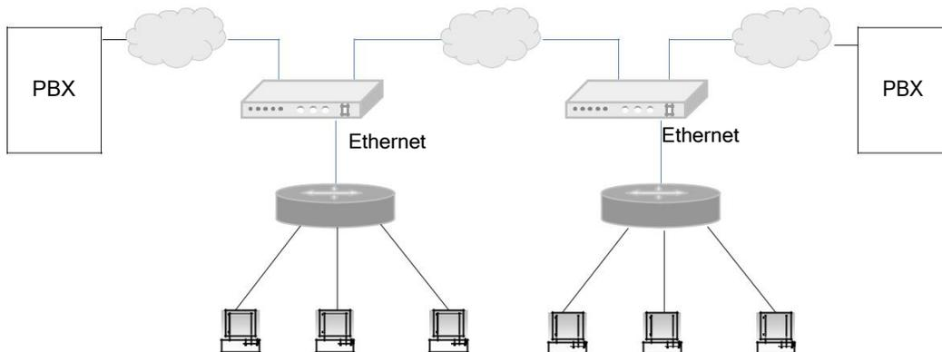
**Note:** When device Ethernet port link with PC, use MDI-X twisted-pair line; link with HUB or Switch, please select MDI twisted-pair line.
